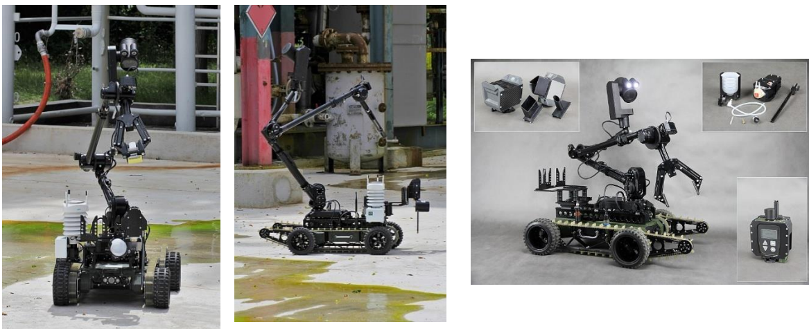
Figure 6. View of GRYF robot provided form PIAP [27]
