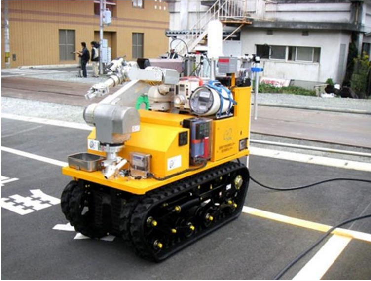
Figure 5. A Monirobo- Japanese vehicle to assist in the recovery of Fukushima nuclear power plant failures [25]
